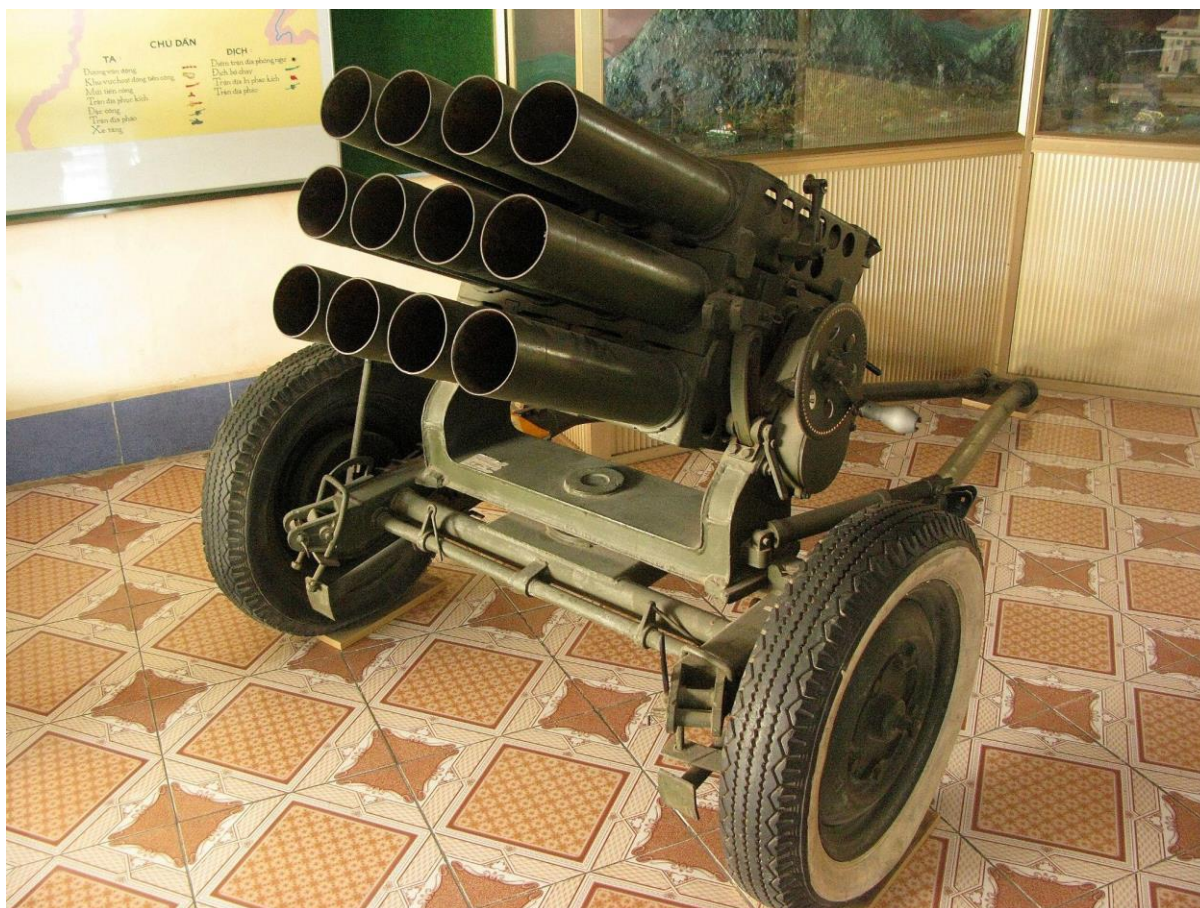
Image (9)- The Type-63, 107mm multiple rocket launcher. Credit .
